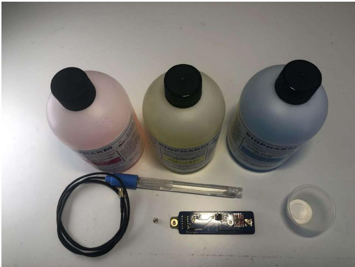
Important Note: If you have older pH standards, you may need to replace them. If you're not able to, or if you're reusing standards for multiple calibrations, consider using a pH meter as a standard, such as the Extech PH100 or equivalent.
