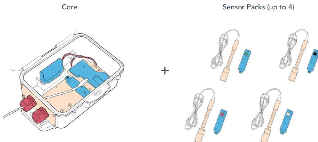
A module's hardware can be changed out in case you need to replace an entire sensor pack or just one component, such as the module board.
